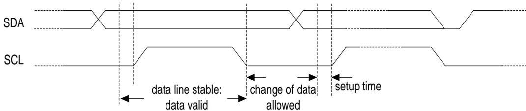
Figure 30. Data and clock timing relation in I<sup>2</sup>C bus
