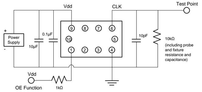
**Figure 7. Clipped Sinewave Test Circuit (OE Function)**
