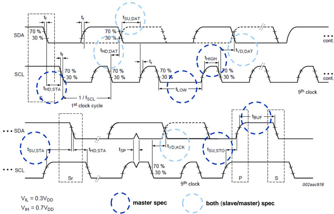
Figure 35. I<sup>2</sup>C Timing Diagram
