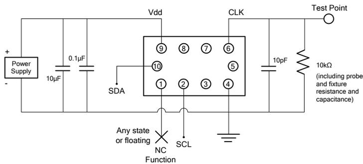
**Figure 13. Clipped Sinewave Test Circuit (I<sup>2</sup>C Control)**
