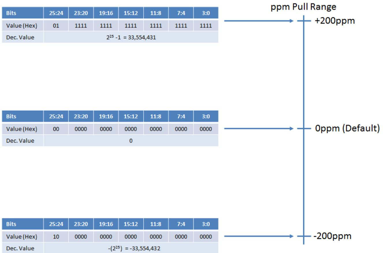
**Figure 29. Pull range and Frequency Control Word**
