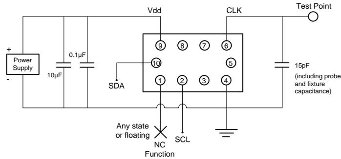
**Figure 12. LVC MOS Test Circuit (I<sup>2</sup>C Control)**
