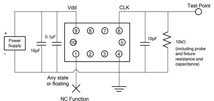
**Figure 11. Clipped Sinewave Test Circuit (NC Function)**
