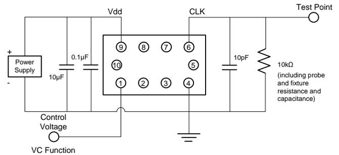
**Figure 9. Clipped Sinewave Test Circuit (VC Function)**
